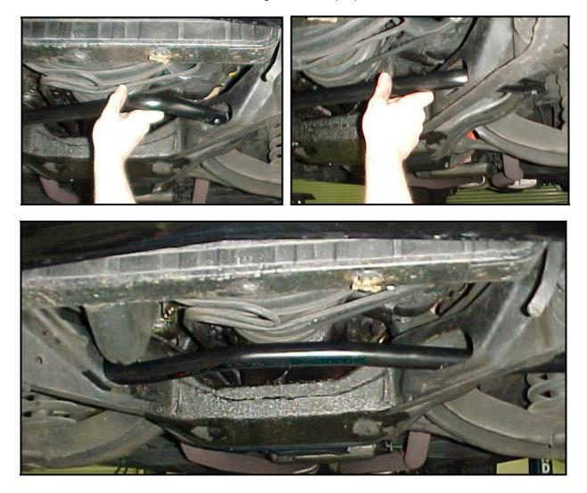
8) Use the grease pack provided to put a heavy coat of grease on the inside of the sway bar bushings. Place the bushings over the bar with the cut in the bushing towards the rear of the vehicle. Push the bushing retainer brackets into place on the bar and bolt them into place <u>using</u> the stock mounting hardware in the front holes only. **Do not** tighten the stock hardware.
