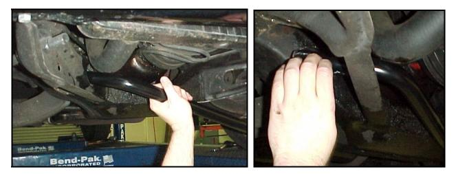
7) Slide the end of the Hotchkis bar between the coil spring and the brake drum in the same fashion as was used to remove the stock bar.
