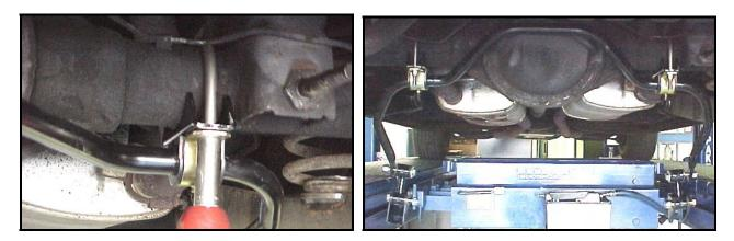
7) Snug down the hardware connecting the end links and brackets to the bar. **Do not** fully tighten the hardware at this stage. You should still be able to rotate the end links without difficulty.
