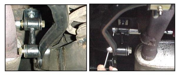
12) Check that all hardware is tight. Use the caps provided to cover the zerk fittings and you're done installing the Hotchkis rear sway bar!
