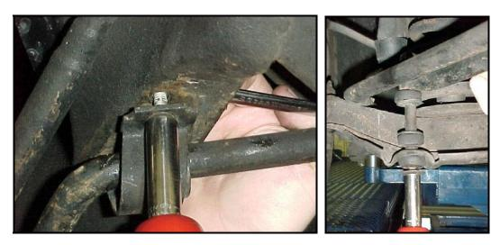
3) Turn the front wheels to point straight ahead. If you jacked up the front of the vehicle, you should now lower the vehicle so that the weight is on the front tires. Slide the stock bar towards the passenger side of the vehicle. *The end of the sway bar should contact the rear edge of the brake drum preventing you from fully removing the sway bar.*
