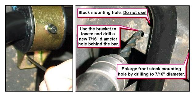
11) Use the 3/8" bolts from **hardware kit #1735** to attach the Hotchkis bar. Drop the bolts down through the drilled out holes in the frame. Start the washers and nylock nuts onto the ends of the bolts. You will use only four of each nut, washer and bolt. <u>DO NOT THROW THE EXTRA</u> <u>HARDWARE AWAY</u>, as it is used for the rear sway bar. Torque the hardware to 35 ft/lbs.
