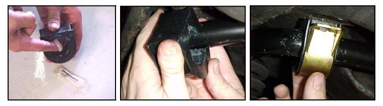
9) With the brackets in place, install the new end links included in the Hotchkis kit at each end of the bar to establish the proper fit of the front bar. *The vehicle weight should be on the front wheels to establish the proper ride position of the sway bar in the vehicle.*
