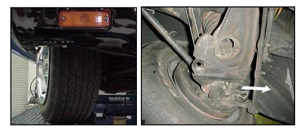
4) Move the sway bar end towards the rear on the passenger side of the vehicle until the opposite end of the bar clears the slot in the frame on the driver's side.
