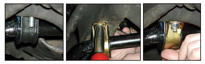
12) Re-place the end links removed in step 10 and tighten them into place. Tighten the end links until the nut meets slightly stiff resistance. The bushings will have a slight bulge when tight.
