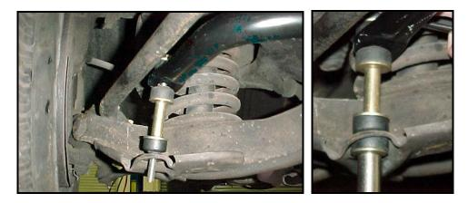
13) Re-check all hardware for tightness. Cover the zerk fittings in the brackets with the grease caps that came attached to the brackets. You are finished with the front sway bar installation
