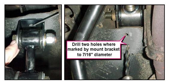
Drill out the holes for the brackets to 7/16" diameter. To accurately determine the location of the holes the end links must not be loose enough to move left or right. Make certain the axle is at its normal driving height for an accurate fit.
