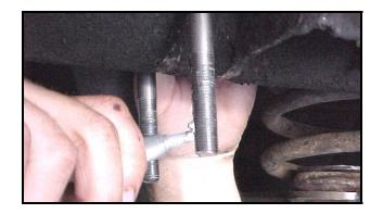
Use the anti-seize provided with the u-bolts to lubricate the threads. Failure to lubricate the threads can destroy the nuts and possibly break the u-bolt or seize the nut in place when tightened.
