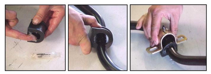
Use the grease provided to apply a heavy coat of grease to the sides of the bushings on the "dog bone" end links. Attach the mounting brackets to the end links using hardware kit #T1712. Attach the other end of the links to the sway bar. Leave the attaching hardware loose.
