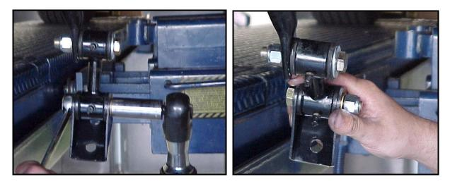
8) Rotate the bar upwards, so that the brackets are resting against the frame. Once the brackets are in place use a scribe or some other tool to mark the center of each hole for drilling.
