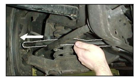
Turn the front wheels to the left until the end of the bar can slide past the rear edge of the brake drum. On some disk brake applications it may be necessary to remove the caliper to allow the sway bar to slide past.
