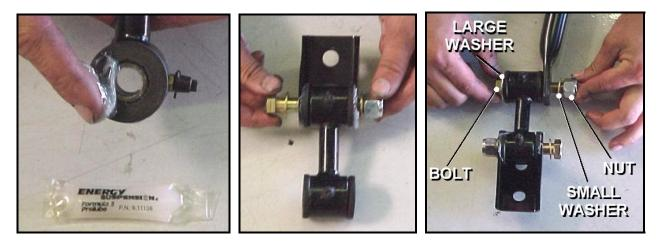
The large washer should be used to contact bushing surfaces and the small washer should be used to contact metal surfaces. This prevents the bolt from pulling through the bushing. You will have 2 large washers and 2 small washers left over. This is extra hardware and may be discarded.
