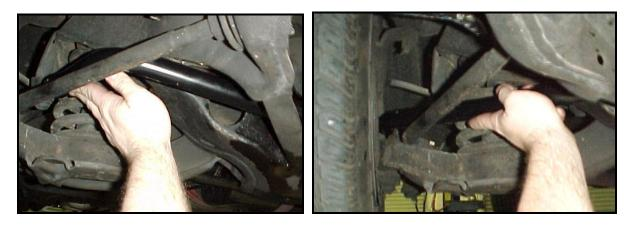
The leading end of the bar should eventually swing into the slot in the frame on the driver's side of the vehicle. The bar will be free moving, but in the proper orientation in the vehicle.
