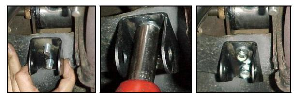
11) Re-attach the end links to the brackets and tighten the hardware into place. Torque the end link hardware to 80 ft/lbs.
