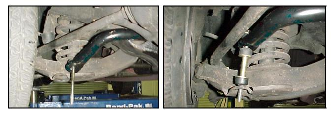
10) With the final position of the bar now determined, you will need a scribe or some other tool to mark with. Mark the center position of the holes for the rear side of the bracket. Remove the brackets, bushings, end links, and stock hardware. Drill the existing front mount hole out to a 7/16" diameter and drill a new rear mount hole at the same size where you marked the frame.
