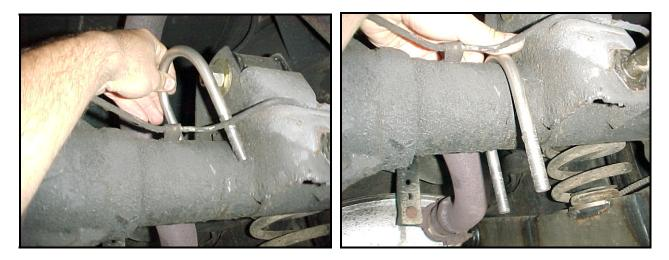
3) Use the grease pack provided to apply a heavy coat of grease to the inside of the sway bar bushings. Place the bushings over the bar. *The split in the bushings should face towards the rear of the vehicle with the bar installed.* Push the brackets over the sway bar bushings.
