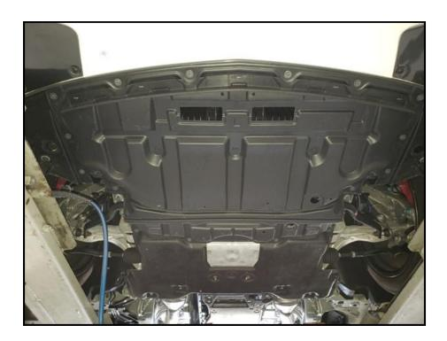
4) Remove the factory plastic undertray from the car by unfastening the bolts and plastic pop clips.
