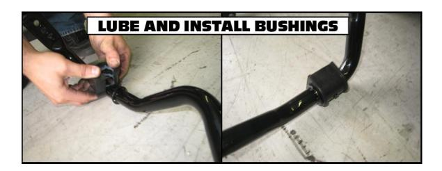
9) Slip the bar into the car over the exhaust and install the endlinks into the end of the bar to help hold it up.
