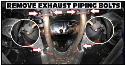
Remove tunnel brace. This will allow the exhaust piping to be lowered and allow easier access to the sway bar. Depending on how high your vehicle is raised, it may be necessary to have something to allow your piping to rest on.
