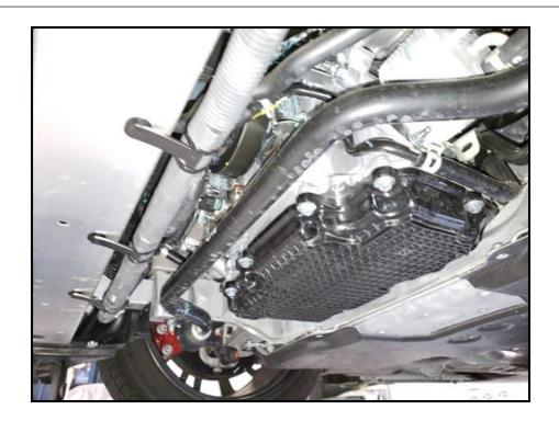
5) Disconnect the endlinks from the sway bar and uninstall the bushings.
