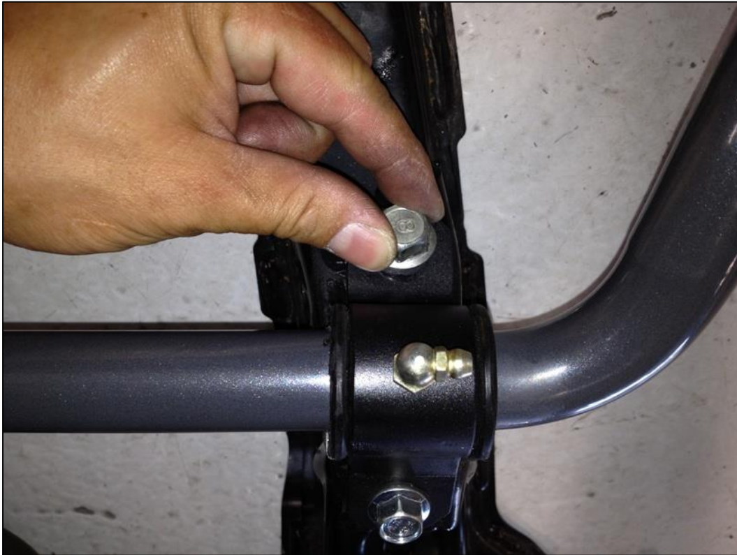
Grease Fitting Points Outwards
