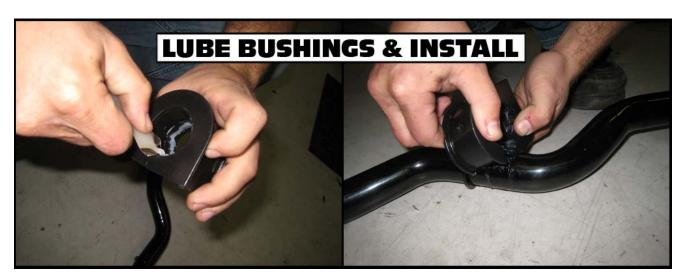
7) Place the new Hotchkis bar in the vehicle and slip the end links into the bar to help support it until you install the bushing brackets.
