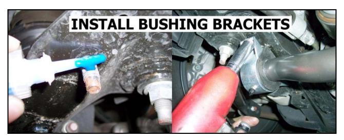
9) Apply thread lock and fully tighten end links to sway bar.
