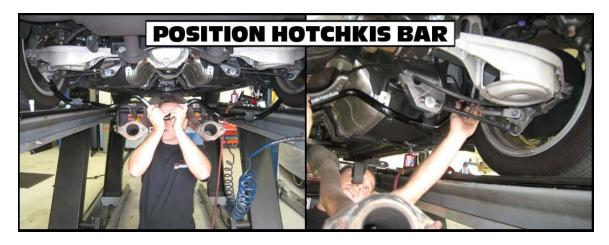
10) Install the Hotchkis brackets over the bushings and using the factory bolts, tighten the bar to the frame.
