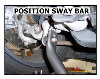
8) Install the bushing brackets making sure thread lock is applied and the zerk fittings are facing outwards.
