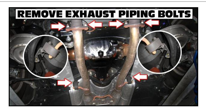
5) Remove tunnel brace. This will allow the exhaust piping to be lowered and allow easier access to the sway bar. Depending on how high your vehicle is raised, it may be necessary to have something to allow your piping to rest on.
