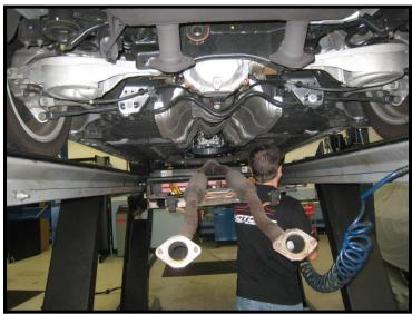
Remove the nuts that hold the endlinks to the bar, leave the end link attached to the sway bar to assist in holding the bar up. Next remove the bushings.
