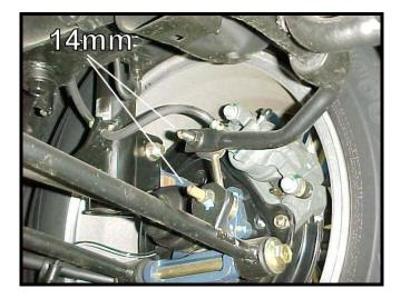
3) Remove the bolts holding the 2 bushing brackets using a 12mm socket. Retain the brackets and hardware for reinstallation. You may discard the stock rubber bushing.
