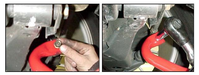
10) Once the end links are connected, you can now fully tighten the bushing bracket bolts to 30ft-lbs
