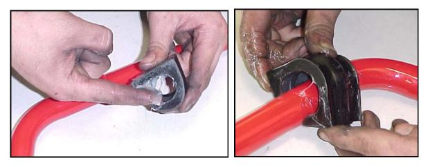
8) Lift the Hotchkis sway bar into position the same way the stock sway bar came out. Use the stock mounting brackets and hardware to secure the new sway bar in place. Do not fully tighten the bracket bolt at this time.
