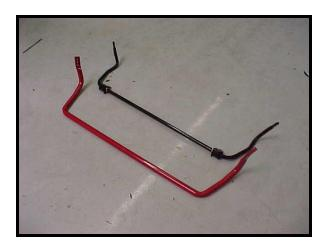
6) Install your new Hotchkis sway bar in the same manner as the stock removal. Just to reiterate, the passenger side end of the bar will be fed up and over the exhaust pipe first. Then the bar can be positioned correctly.
