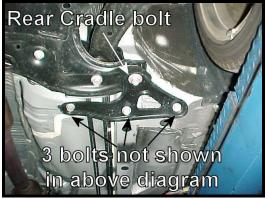
4) Use a 14mm Socket to remove the 3 Nuts and 2 Bolts that secure the lower engine mount to the cradle. Retain all hardware for re-installation.
