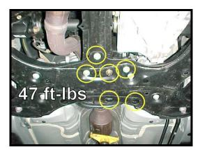
5 – Install the 4 nuts to secure the steering rack to the cradle. Torque to **45 ft-lbs**.
