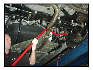
7) Lube the inside hole of your new Hotchkis polyurethane bushings and install the bushings on to the bar.
