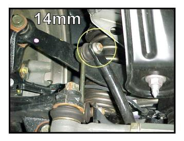
3) Remove the nut and bolt for each side subframe mount using a 14mm socket. You may discard this hardware.
