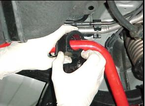
8) Place the provided bushing bracket over the bushing and set the sway bar into it's proper position. Install the provided nut and bolt & flat cut washer to secure the bracket to the frame of the vehicle.
