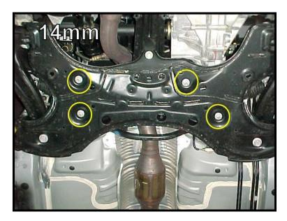
8) With all the nuts & bolts removed the cradle should droop loosely enough to reach the sway bar mounted to the top rear portion of the cradle. Use a 14mm socket or wrench to loosen and remove the four bolts holding the stock sway bar in place. Remove the stock sway bar, bushings and brackets. Retain the stock bolts for re-installation.
