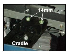
7) Remove the 4 nuts that secure the steering rack to the cradle. It's suggested that you use an impact wrench for easier removal.
