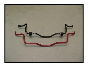
10) Re-install your new Hotchkis sway bar in the same manner as the stock sway bar removal. Install using the included Hotchkis polyurethane bushings and brackets. It's a good idea to install the bushings and brackets after the bar is in position. Lube the inside of each bushing with the provided grease. Use bushing prt # 5339.
