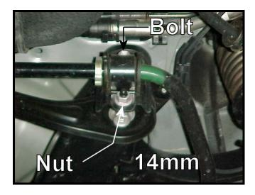
4) Remove the subframe bushing and bracket to ease the removal of the bar from the vehicle. You may discard the old bushing and bracket. Gently pull the sway bar towards the front of the car and the driver side end should be free to drop out.
