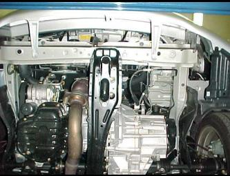
6) Next, remove the 2 bolts that secure the cradle bridge bracket to the radiator support.
