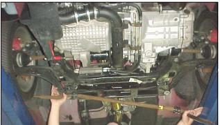
4. Now you're ready to grease the new bushing with the provided grease. Then place the bushing over the bar. Now start the bolts for the mounts into the frame.
