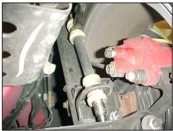
3. Now remove the sway bar mounts from the frame and completely remove the bar.
