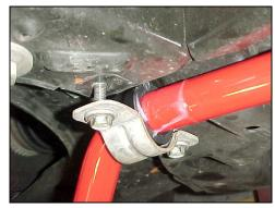
5. Now install the new end links and tighten using a 14mm socket and wrench. Lube all of the end link bushings with the provided grease.
