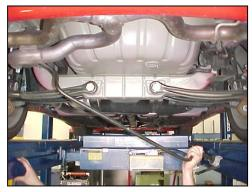
4.) Now you're ready to grease the new bushing with the provided grease. Then place the bushing over the bar followed by the bracket.
