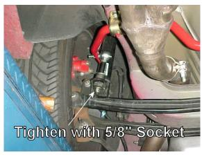
7.) Now you can tighten the sway bar frame mounts. Then tighten up the jam nut on the end link.
