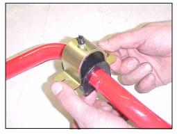
5.) Go ahead and start but don't tighten the sway bar frame mounts.
