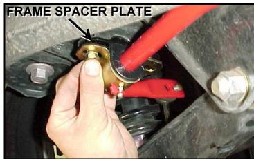
Use a 12mm socket or wrench to tighten the sway bar mounting brackets. Torque the hardware to 30ft/lbs. Use a 14mm wrench and 5mm Allen wrench to tighten the end link sway bar. Torque the end link hardware to 25ft/lbs.
