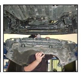
3) The stock front sway bar should now be exposed. Use a Phillips screwdriver to remove the side splashguards. Remove the retainer screws on each side and retain all hardware and splashguard pieces.
