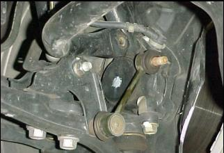
5) Use a 12mm socket or wrench to loosen and remove the bolts holding the sway bar bushings and bushing retainer brackets in place. The front sway bar should now just drop out. Remove the stock front sway bar. Keep the stock hardware for later re-installation. The stock brackets, bushings, and sway bar will not be re-used.
