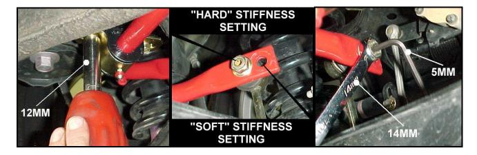
As was shown on the front bar, the stiffness of the rear bar is determined by the hole used with the end link. The hole nearest the ends is the "soft" setting and the hole towards the middle is the "hard" setting.
