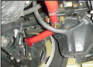
9) Install the stock end links into the ends of the Hotchkis bar. Note the position of the hole. The hole closest to the end of the bar effectively lengthens the bar for the "softest" stiffness setting. The hole closer to the center of the bar effectively shortens the bar and is the stiffest setting. Tighten the stock nut on the end link with a 5mm Allen wrench and 14mm wrench. Torque the hardware to 25ft/lbs.
