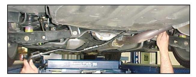
Use the grease pack provided to apply a thick coat of grease to the inside of the sway bar bushings. Slide the bushings over the bar and place the bushing retainer brackets over the bushings. You might find it easier to install the bushings and brackets after the Hotchkis bar is in place on the vehicle due to exhaust clearance of the bar itself.
