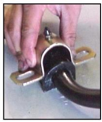
Lift the Hotchkis bar into the vehicle over the exhaust in the opposite way in which you removed the stock bar. Slide the frame spacer plate into place for the bushings to rest against as shown. Use the stock hardware to mount the bushing brackets and spacer plate to the sub-frame.
