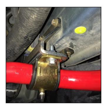
A properly installed bar will have the middle "hoop" of the bar closest to the ground when looking at it from the front.
