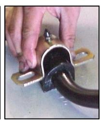
8) Lift the Hotchkis sway bar into position the same way the stock sway bar came out. Use the new mounting brackets and stock hardware to secure the new sway bar in place. The end of the bar on the driver's side should slide through the hose as shown.
