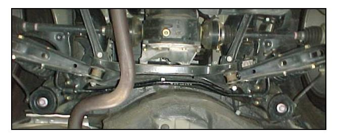
Use a 14mm wrench and 5mm Allen wrench to loosen and remove the end links from the sway bar. Use a 12mm socket or wrench to loosen and remove the bolts holding the sway bar bushing brackets. Retain all stock hardware. You may discard the stock sway bar, bushing, and bushing retainer brackets.
