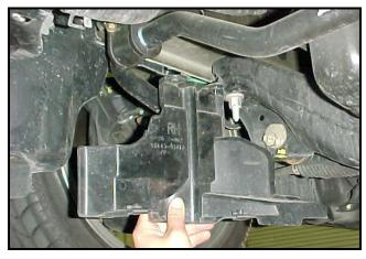
4) Unbolt the stock end link from the sway bar on each side. Use a 14mm wrench and a 5mm Allen wrench to remove the nut from the end link and pull the end link out of the sway bar. Retain the hardware for re-installation.
