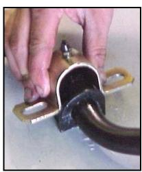
6) Lift the Hotchkis bar into the vehicle over the exhaust in the opposite way in which you removed the stock bar. Slide the frame spacer plate into place for the bushings to rest against as shown. Use the new Hotchkis hardware to mount the bushing brackets and spacer plate to the subframe.
