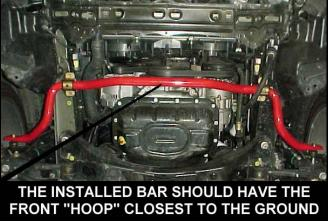
10) Re-check all attaching hardware for tightness. Re-install the splashguards on the sides and main splash-pan underneath using the stock hardware. Use a jack to remove the jack stands.
