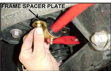
7) Use a 12mm socket or wrench to tighten the sway bar mounting brackets. Torque the hardware to 30ft/lbs. Use a 14mm wrench and 5mm Allen wrench to tighten the end link sway bar. Torque the end link hardware to 25ft/lbs.
