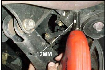
4) The stock sway bar should now be loose and can drop out starting at the driver's side and slide out over the exhaust. The Hotchkis bar will install in the same manner as the stock one.
