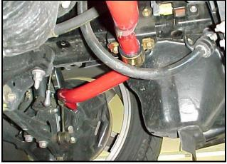
8) Install the stock end links into the ends of the Hotchkis bar. Note the position of the hole. The hole closest to the end of the bar effectively lengthens the bar for the "softest" stiffness setting. The hole closer to the center of the bar effectively shortens the bar and is the stiffest setting. Tighten the stock nut on the end link with a 5mm Allen wrench and 14mm wrench. Torque the hardware to 25ft/lbs.
