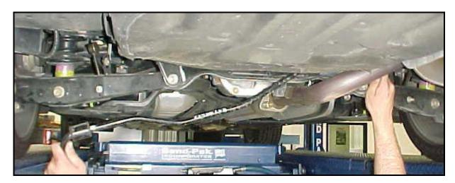
5) Use the grease pack provided to apply a thick coat of grease to the inside of the sway bar bushings. Slide the bushings over the bar and place the bushing retainer brackets over the bushings. You might find it easier to install the bushings and brackets after the Hotchkis bar is in place on the vehicle due to exhaust clearance of the bar itself.
