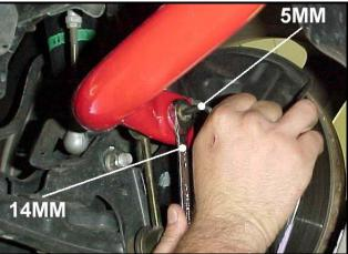
9) With the end links tight you can secure the bolts holding the sway bar in place. Use a 12mm socket or wrench to tighten the bolts. Torque the hardware to 30ft/lbs. A properly installed bar will have the middle "hoop" of the bar closest to the ground when looking at it from the front.
