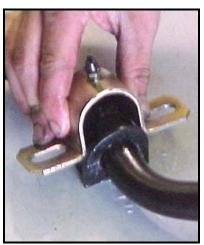
7) Lift the Hotchkis sway bar into position the same way the stock sway bar came out. Use the new mounting brackets and stock hardware to secure the new sway bar in place. The end of the bar on the driver's side should slide through the hose as shown.
