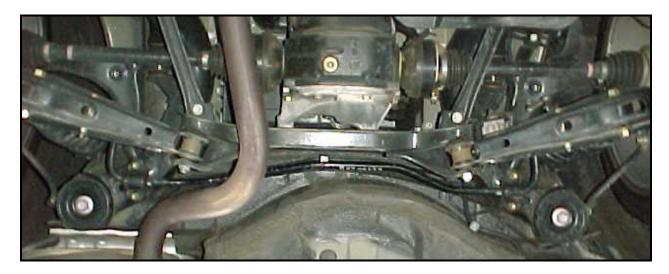
3) Use a 14mm wrench and 5mm Allen wrench to loosen and remove the end links from the sway bar. Use a 12mm socket or wrench to loosen and remove the bolts holding the sway bar bushing brackets. Retain all stock hardware. You may discard the stock sway bar, bushing, and bushing retainer brackets.
