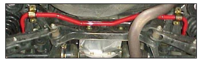
8) Re-check the hardware for tightness. Cover the zerk fittings with the caps attached to the brackets. Use the jack to remove the jack stands and you're finished installing your Hotchkis Tuning sway bar set.
