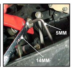
As was shown on the front bar, the stiffness of the rear bar is determined by the hole used with the end link. The hole nearest the ends is the "soft" setting and the hole towards the middle is the "hard" setting.
