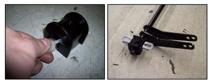
Position the sway bar onto the truck as shown. <u>The sway bar lever arms point</u> towards the rear. Use the hardware from bag #17118-1 to mount the bushing bracket to the frame. The longer bolts (1.25") are for the front hole and the shorter bolts (1") mount the rear holes. Center the bracket so that the holes are in the middle of the bracket slots. Fully tighten the bolts.
