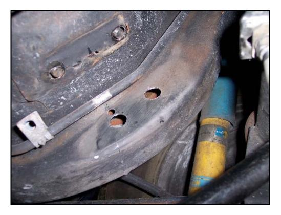
Insert the reinforcement plate with the 2 tubes welded to it into the frame rail. Use a vise clamp to secure the plate onto the frame rail. Drill the outer wall of the frame rail with a  $\frac{1}{2}$ " drill bit. The reinforcement tubes will act as a guide for you to drill. So when you are finished, you will have two  $\frac{3}{4}$ " holes on the inside of the frame rail and two  $\frac{1}{2}$ " holes on the outer sided of the frame rail.
