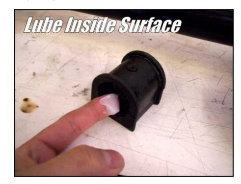
2R. Take the bushings and grease the inner surface with the included white silicon grease.
