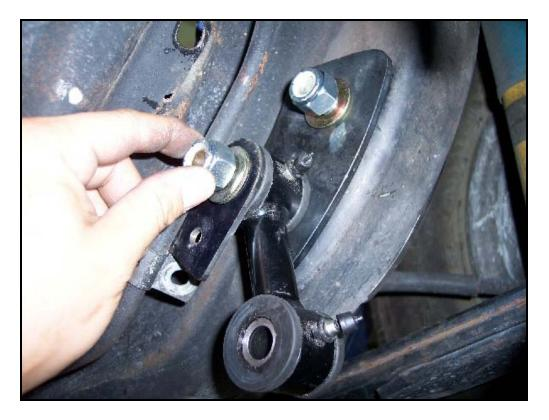
Line up the mounting tab with the line bracket you just installed. Use the provided 5/16" bolt and washer to secure the mounting tab to the line bracket. (hardware kit **#1757**) Make sure the  $\frac{1}{2}"$  Nut is not too close to the fuel line.
