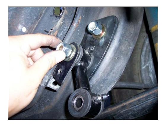
Line up the mounting tab with the line bracket you just installed. Use the provided 5/16" bolt and washer to secure the mounting tab to the line bracket. (hardware kit **#1757**) Make sure the  $\frac{1}{2}$ " Nut is not too close to the fuel line.
