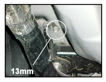
6) Support the rear axle pumpkin housing with a jack. Try to use wood or a rubber pad to cushion the contact point of the jack and housing. Remember the jack stands should still be supporting the rear of the vehicle.
