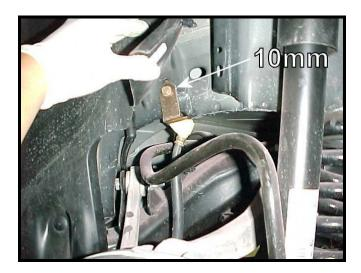
Next, you will need to drop the exhaust system for clearance. Unbolt the mid-brace removing the 4 bolts using a 13mm socket. Spray the rubber hangers in the picture with WD-40 and slide the rubber hanger off the exhaust support. Unbolt the remaining rear hangers using a 13mm socket. Be careful, for the exhaust will drop down once these bolts are out.
