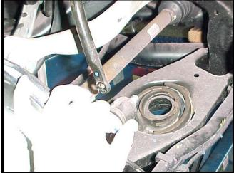
10) Unfasten the 2 bolts securing the subframe mounts using a 15 wrench. Retain the bolts for reinstallation. You may discard the stock bushing brackets.
