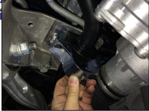
Install the Hotchkis saddle brackets using the included washers.
