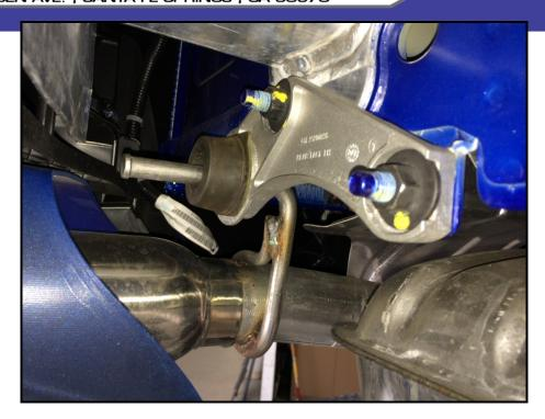
Pop off the (4) remaining rubber hangers. Spraying these with WD-40 will help aid in disconnecting these.
