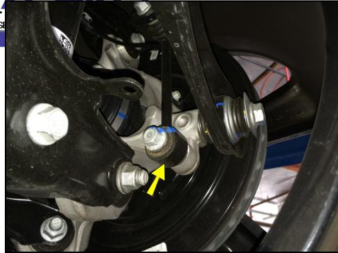
5R Fish the OE rear sway bar out of the car. Start by rotating the lever arms rearward and then pull the bar out toward one of the wheels.
