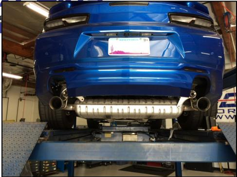
3R Unbolt the saddle brackets that hold the bushings in place.
