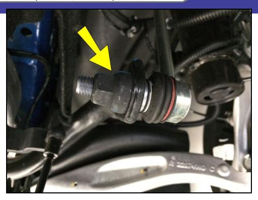
5F Unbolt the saddle brackets that hold the bushings in place. Remove the oe front bar.
