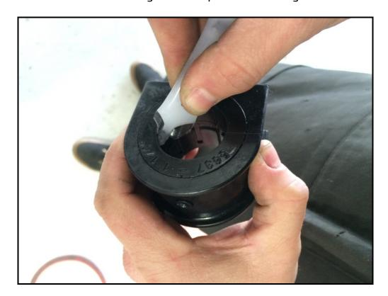
Position the Hotchkis bar onto the car and Install the Hotchkis polyurethane bushings onto the bar.
