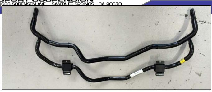
7F Lube the Hotchkis front bushings with the provided silicon grease.
