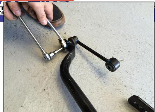
7R Lube the Hotchkis rear bushings with the provided silicon grease.
