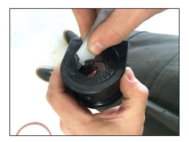
Position the Hotchkis bar onto the car and install the bushings onto the bar. It helps to insert the end links into the holes to help hold up the bar
