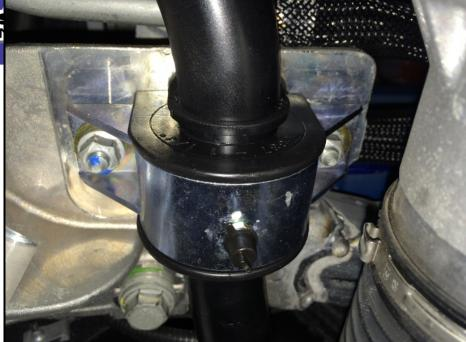
8F Completely fasten the end links to the sway bar ends. You have (3) holes to choose from. The holes closest to the end are the softest setting. We suggest using the stiffest holes to start.
