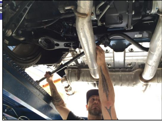
6R Set the oe bar next to the Hotchkis bar for comparison and position/orientation. Transfer over the oe end links from each end onto the Hotchkis bar. You have (3) holes to choose from. The holes closest to the end are the softest setting. We suggest using the softest holes to start.
