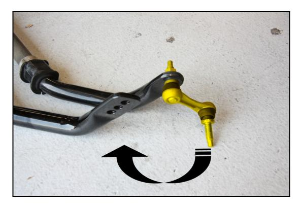
5R Lube the Hotchkis rear bushings with the provided silicon grease.
