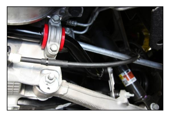
7R Lower vehicle to the ground and you are complete with the rear sway bar install.
