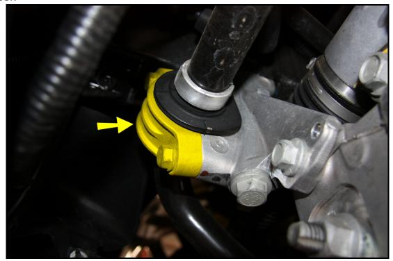
6F Set the oe bar next to the Hotchkis bar for comparison and position/orientation. Transfer over the oe end links from each end onto the Hotchkis bar.
