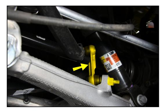
3R Unbolt the saddle brackets that hold the bushings in place. Remove the oe rear bar.
