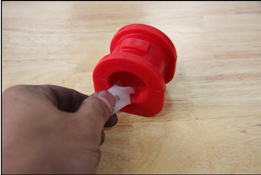
Position the Hotchkis bar onto the car and install the bushings onto the bar.
