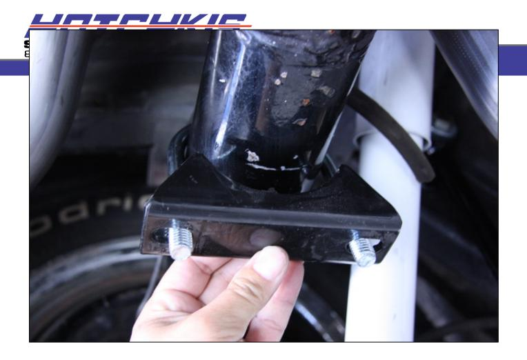
Rotate the sway bar up towards the axle until the u-bolt lines up with the busing bracket. Install the washer and nylock nut onto the u-bolt. Snug up this nuts, but do not fully tighten at this time. Make sure both left and right axle brackets are parallel with each other. Also, try to get the axle brackets level to the ground. If the drop links are at a severe angle, it is ok to adjust the axle brackets to straighten out the drop links.
