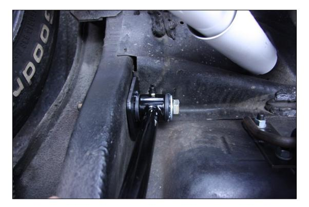
Install the mount plate, washer & nut on the other side of the frame rail. Do not fully tighten at this time.
