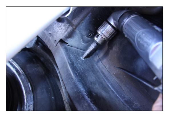
Insert the plate with tube into the 3/4" hole. Use a 1/2" drill bit and drill the hole using the plate with tube as a guide. Repeat this for the other side.
