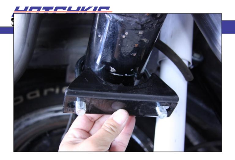
Rotate the sway bar up towards the axle until the u-bolt lines up with the busing bracket. Install the washer and nylock nut onto the u-bolt. Snug up this nuts, but do not fully tighten at this time. Make sure both left and right axle brackets are parallel with each other. Also, try to get the axle
