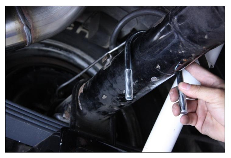
With the u-bolt in place, position the axle bracket up to the axle tube.
