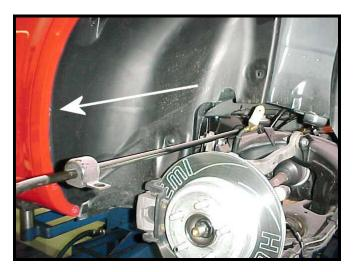
12) Compare the stock bar to your new Hotchkis bar for orientation purposes. Lube the bushings with the provided grease and place them onto the bar.
