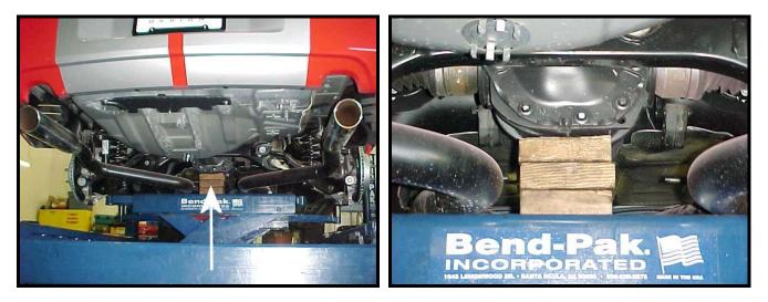
7) Once the axle is supported, you can unbolt the 4 bolts that secure the rear cradle to the frame using a 18mm socket.
