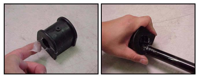
13) Feed your new Hotchkis sway bar into the sway bar location in the same manner as removal. Make sure the bar is oriented as shown in the picture. Place the provided bushings mounts over the bushings and make sure the 90° zerk fittings are facing outboard. Fully tighten the stock bracket bolts.
