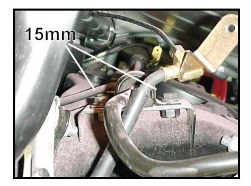
11) The bar should be free to come out. The only obstacle when removing the sway bar is the brake lines may be in the way. If so, carefully push the bar around the brake lines.
