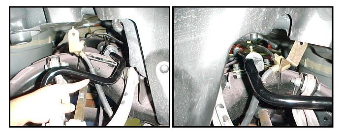
14) Reattach the endlinks to the sway bar in the same manner as removal. Fully tighten all hardware
