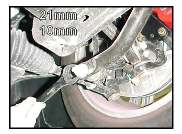
5) Apply a healthy amount of the provided grease to the new Hotchkis polyurethane bushings. One pack per bushing should be used. Your kit comes with 5 packs of grease (2 for front, 1 for rear, 2 for front after 6-12 months). Your front bushings will need to be maintained with grease every 6-12 months depending on your driving conditions. We include 2 extra packs for this purpose.
