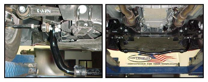
7) Install the subframe mounts back onto the vehicle. Fully tighten all hardware at this time (including the endlink bolts!)
