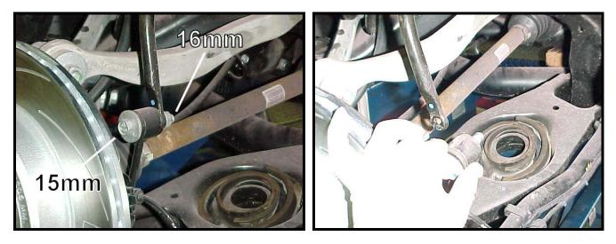
10) Unfasten the 2 bolts securing the subframe mounts using a 15 wrench. Retain the bolts for reinstallation. You may discard the stock bushing brackets.
