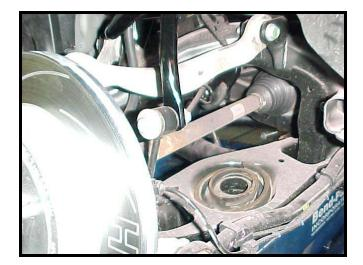
15) Once everything is in place, raise the rear axle into position. Do not raise all the way up! You will still need some wiggle room to line up the cradle bolt holes. Start each bolt by hand to ensure proper threading. Once thread started, fully tighten the cradle bolts using a 18mm socket.
