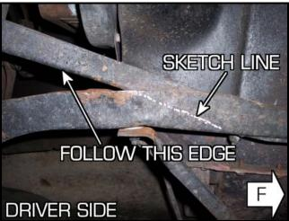
Your Hotchkis kit includes bushing bracket reinforcement plates, which will be installed on the inside of the frame rail. When measuring out where to drill the holes, your main goal is to position the holes as far forward without contacting the inner frame rails. See picture for more details. Make sure the 2 holes are parallel with the length of the car. Drill the holes using a 7/16" drill bit. Remember to always wear safety glasses when drilling.
