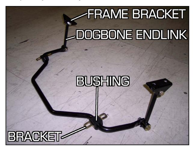
You will also need to grease the outside surface of the dogbone end link bushings. Install the end link onto the sway bar ends as shown in the picture. Use the hole closest to the end for installation purposes. Next, install the frame bracket onto the other end of the end link. The bolts do not need to be fully tight at this time, but they should be snug.
