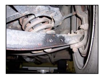
Install the end link bracket onto the lower control arm with the supplied bolts.
