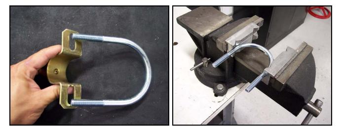
The U-bolt should just pass through the widest section of the bushing bracket slots. Try to not clamp down the vice too much, you don't want to over bend the U-bolt.
