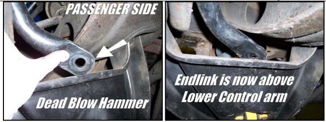
Once the anti-roll bar end is above the lower control arm, you can easily slide it into position.
