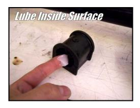
10F. Install the bushing on the new Hotchkis bar. Make sure the split on the bushing faces the front when the bar is installed in the vehicle. Look at the placement of the original stock bushings on the stock bar for quidance.
