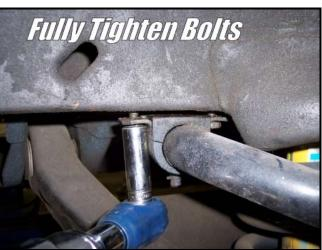
12F. It is best to tighten the endlinks with the suspension at ride height. To achieve this, simply reinstall the wheels and drive the car onto some floor ramps. These can be found at your local auto store. Now, with the car at ride height and on the floor ramps you can crawl underneath the car and fully tighten the endlinks. Tighten the endlinks until the bushings are squeezed just enough that their diameter is just larger than the supporting washer.
