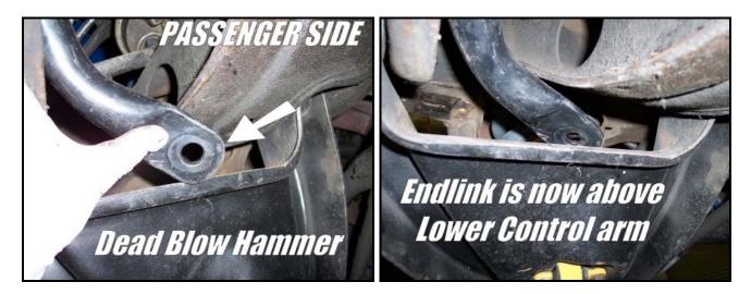
Once the anti-roll bar end is above the lower control arm, you can easily slide it into position.
