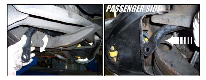
At this point the sway bar will need a little force to get into position. Take your trusty dead blow hammer and hit the anti-roll bar end as shown in the picture below. It won't take too much to pop it into place.
