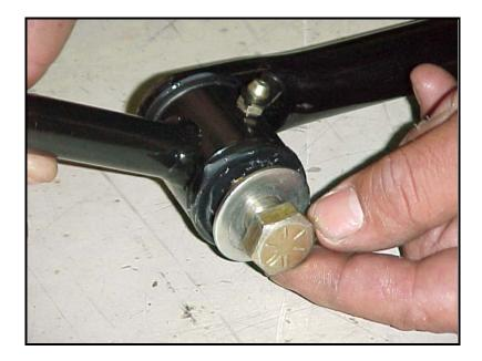
17R. Slide the other end of the dog bone style end link up in between the brackets on the chassis brace. Check for exhaust clearance in this area. If necessary, you may have to have the exhaust pipes re-bent to provide clearance for the new sway bar assembly. Any competent exhaust shop can handle this modification easily. If clear, use the shorter (2.75") bolt with a small washer on each side of the bracket to complete the assembly and fully tighten.
