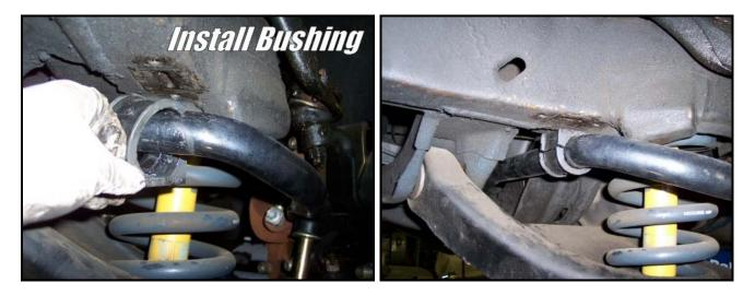
11F. Place the greasable bracket over top the bushing and secure them with the stock bolts. You may fully tighten these bolts at this time.
