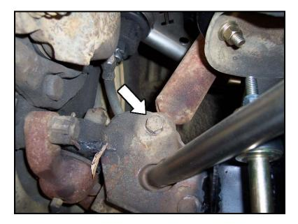
e) Remove the lower ball joint/steering arm from the spindle. There are 2 castle nuts that hold it in place.
