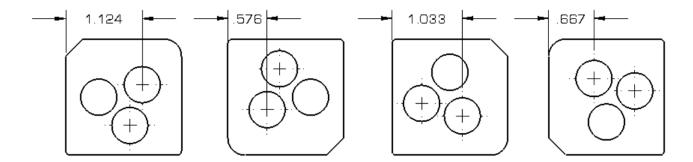
The Hotchkis plates have a unique shape with a chamfer on one corner and a large radius on another. The last (2) corners are sharper corners. This shape allows for easy identifying to insure the clocking is the same for each pair of plates. Just remember chamfer goes with chamfer and radius goes with radius. Your holes will always line up.
