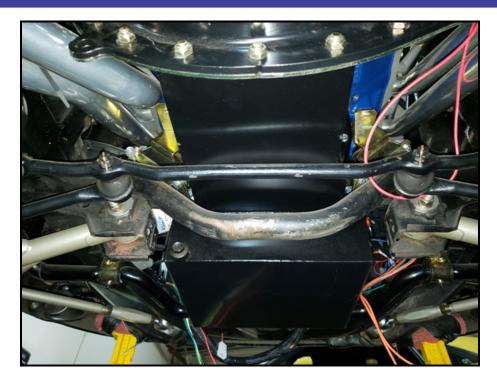
It is held in by (2) bolts, one on each frame rail. Remove these bolts and the brace will be disconnected from the vehicle.
