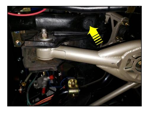
4 Install Lower Control Arm Lock-Out Plates
