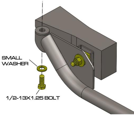
Make sure to tighten the frame bolts and lower control arm nylocks a little at a time. Once all are snug, fully tighten the lower control arm nylocks first then finish with the frame bolts.
