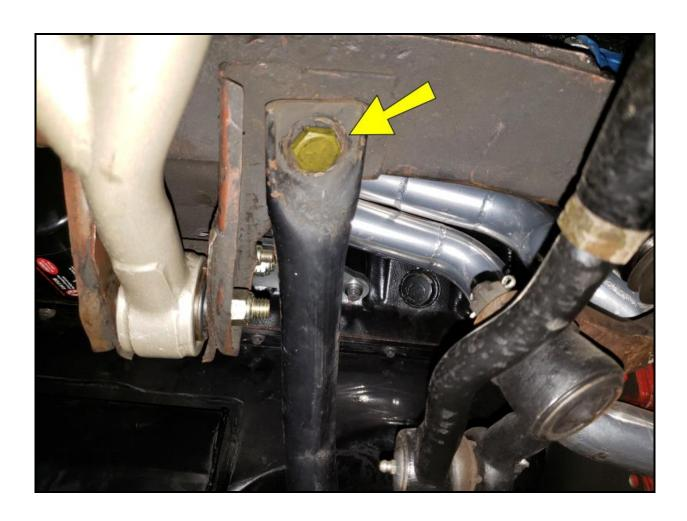
It is held in by (2) bolts, one on each frame rail. Remove these bolts and the brace will be disconnected from the vehicle.
