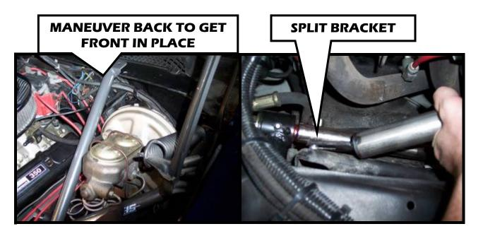
4. Put in the bolt that attaches the Handle Bar Brace to the fender bracket. Only tighten this bolt until it is snug, still allowing the Handle Bar Brace to move slightly.
