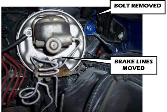
NOTE: Brake lines may need to be pushed out of the way to make room for Handle Bar Brace.
