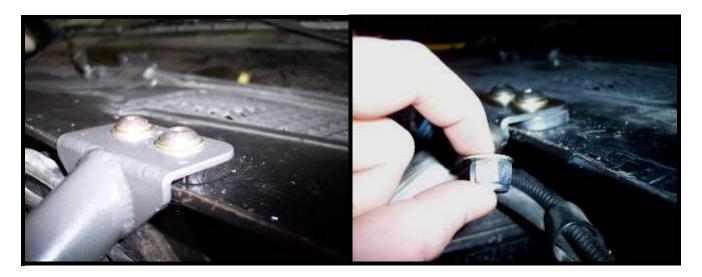
8. Tighten top firewall mount bolts and the fender bracket bolt.
