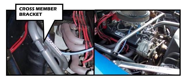
9. Now tighten the fender/firewall bracket end first and then tighten the A-arm bracket. Your Handle Bar Brace system is now ready to go.
