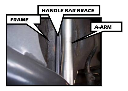
6. Put the A-arm bolts back into place, making sure they pass though the Handle Bar Brace bracket. Using the hardware provided, bolt the Brace to the fender/firewall hole.
