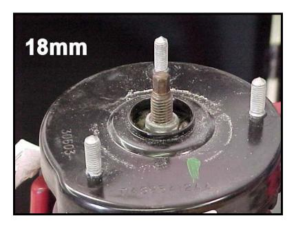
9) Remove the top hat, stock bumpstop, and stock spring at this time. Sometimes the bumpstop is pressed into the top hat, in which case, remove the stock bumpstop from the top hat boot.
