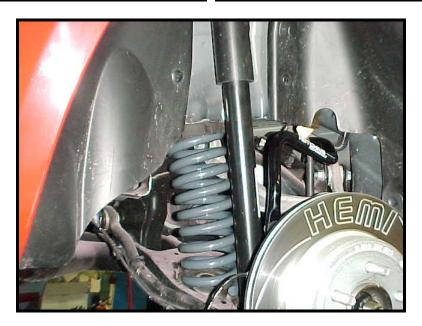
Once everything is in place, raise the rear axle into position. Do not raise all the way up! You will still need some wiggle room to line up the cradle bolt holes. Start each bolt by hand to ensure proper threading. Once thread started, fully tighten the cradle bolts using a 18mm socket. Torque bolts to 133 ft·lbs.
