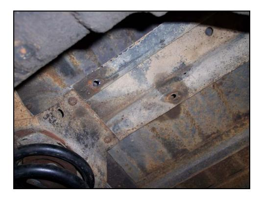
Next, remove the lower shock mounts by undoing the large u-bolts holding the rear axle to the trailing arms. The lower mounts should be loose from the arms. You may discard the upper and lower mounts.
