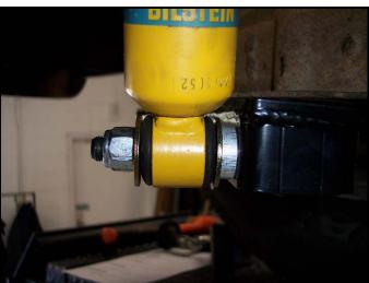
New hardware is also provided for the upper mount. The Hotchkis upper mount has 2 adjustment holes. The hole toward the rear is the stiffer shock setting. Once the shock is in place, fully tighten all shock hardware.
