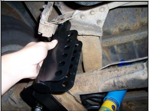
Take the  $\underline{\text{shorter}}$  adjustable bar and install it on the  $2^{\text{nd}}$  or  $3^{\text{rd}}$  hole on the driver side mount bracket. Grease bushing surface with provided lube.
