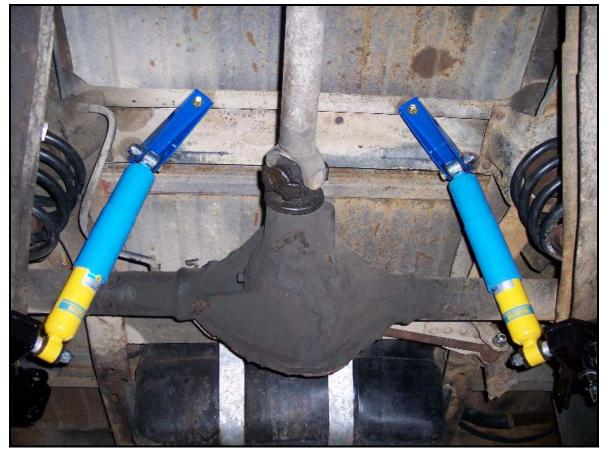
Lower the lifting jack from the trailing arms and you are now finished with the rear shock installation.
