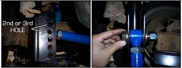
Attach the passenger side frame bracket to the bar using the included hardware.
