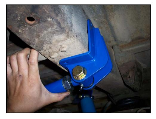
Mark the passenger side frame rails to record all of the holes for the bracket.
