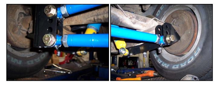
Once all of the suspension members are in place, measure the distance between the inside of the rear tires and the wheel wells. Adjust the track bar (lower one) in or out to equalize the tire gap. Once adjusted, fully tighten all of the hardware.
