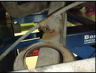
3) Unbolt the shock from the rear axle, and pull it clear of the mounting stud.
