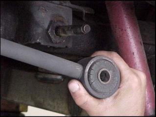
4) Match the Hotchkis panhard rod to the stock Chevy panhard rod. To adjust the Hotchkis panhard rod, loosen then jam nuts at each end. Rotate the middle section to shorten or lengthen the bar. DO NOT rotate the ends of the rod individually as this will affect the maximum and minimum adjustment of the bar.
