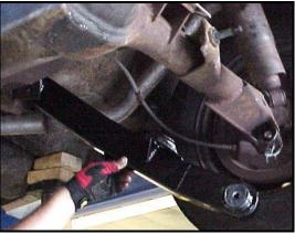
7) Install the arm into the mounting locations on the frame and axle. Use the hardware kit provided and the original shock mount stud to secure the Hotchkis trailing arm in place. **Do not** tighten the hardware until both ends of the arm have been connected to the axle and frame.
