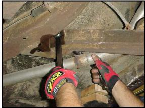
The hardware at the rear of the arm is easily accessed and should be removed. Retain the stud for later use. With all the hardware removed the stock arm should drop out of place.
