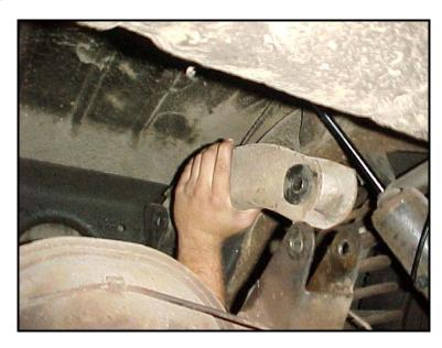
3) Check the stock arm mounting hole center-to-center measurement. The stock arm length should match the length of the Hotchkis upper arm center-to-center measurement.
