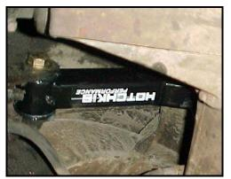
With the arm(s) in place, determine if any pinion angle adjustment is necessary. For stock vehicles no adjustment should be required. If the pinion angle needs to be adjusted downwards, the arm length needs to be shortened. If the angle needs to be adjusted upwards, the arm length should be extended.
