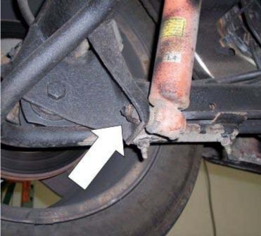
5. Remove the rear swaybar from the lower trailing arms. Trailing arm mounts: 15mm socket/wrench for nuts
