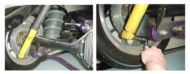
5) Using the jack placed under the differential, raise the rear suspension to its approximate ride height. The braces are generally easier to install with the rear axle at its normal ride height position to the frame.
