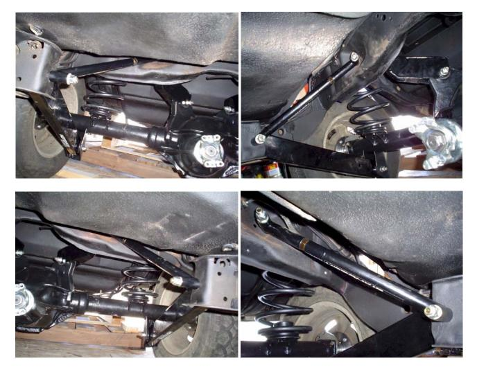
**NOTE:** For 78-88 models (part #1401) the curved section fits next to the lower trailing arm between the rear seat pan and the frame cross-member as shown in the photos below.
