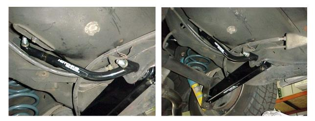
9) Adjust the length of the brace as necessary. Loosen the jamb nut on the brace with 15/16" wrench to allow the head to move. Rotate the head clockwise to shorten the brace or counter-clockwise to lengthen the brace until it fits over the ends of the bolts. The brace ends should fit almost flush to the frame with the bolts fully extended through the ends.
