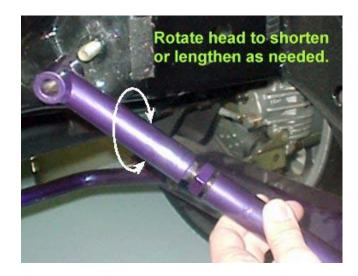
**YOU WILL NOT,** be able to determine if you have the right brace length until you have fully extended the bolts and the brace fits without causing the hardware to bind.
