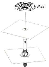
POSITION BASE ON TOP OF THE HOOD. CENTER THE BASE WITH THE HOLE.
