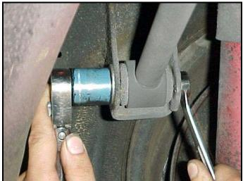
3) Remove the stock panhard rod. Rotate the top end of the bar out of the bracket on the frame and then pull the bar off the stud on the axle.
