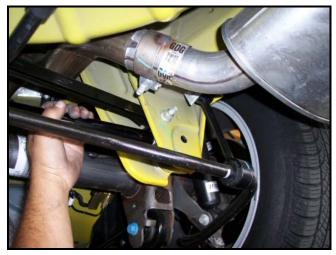
An adjustable panhard rod is used to give the owner the ability to laterally center the rear wheels with the chassis. This is usually needed with lowered vehicles.
