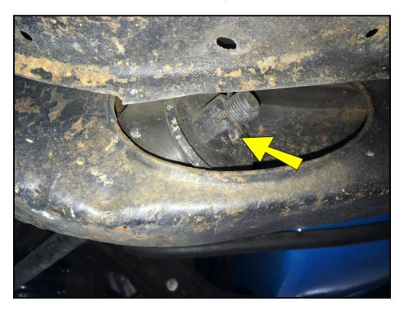
Unbolt the castle nut and remove the strut rod.
