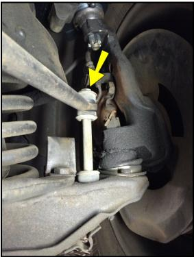
3 *Unbolt the Strut Rod From the LCA* Unbolt the (2) nuts holding the strut rod to the LCA (lower control arm).
