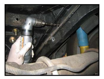
12R. Place chassis brace back into place and mark the remaining 4 holes for drilling as shown below. After marking the holes, remove brace and using a 7/16" drill bit, drill the holes.
