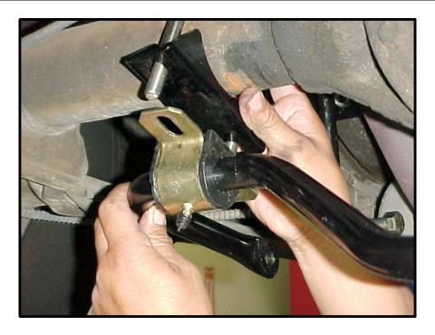
8R. Remove the screw and clip that holds the fuel line located on the frame rail of the passenger side to allow for the chassis brace to slide into place. '68 cars may need to drill out rivet style line tabs.
