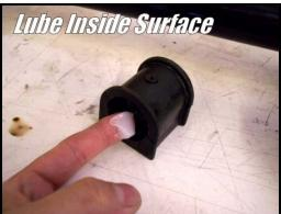
4R. Install the bushings on the bar. (4) Place the bracket over top of the bushing. (5)
