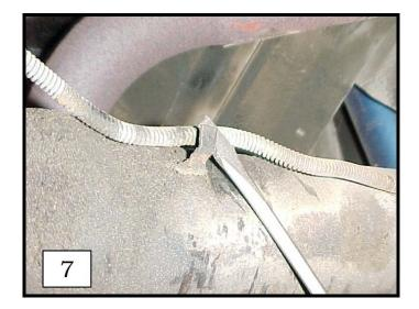
7R. Install the U-Bolts on the axle and slip the axle bracket over the U-Bolt on the bottom side of the axle. Use masking or duct tape to secure them. Place the sway bar assembly under the axle and slip the U-bolt legs through the sway bar brackets. Place washers and nylock nuts on the U-Bolt. Snugly fasten the nylock nuts a bit, but do not fully tighten at this time.
