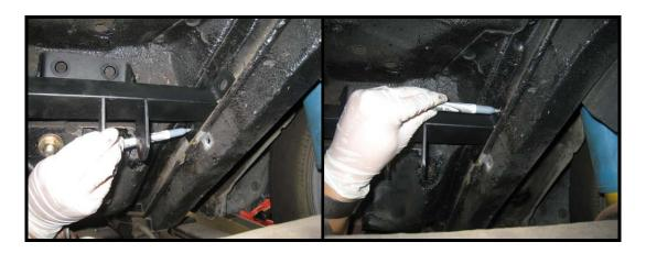
11R. Remove the chassis brace and using a 7/16" drill bit, drill the 4 holes that you just marked.
