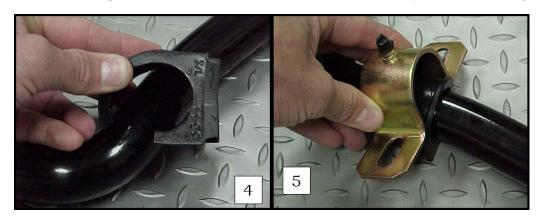
5R. After you determine there's enough clearance for the bar, note the approximate location of the sway bar axle bushings.
