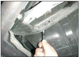
Once you have removed the inside hardware, remove the arm and place it on a flat surface. Take one of the HSport arms and place it over the stock piece and line up the sleeves at either end. This ensures that the HSport arms are in fact at the stock lengths. It will also serve as a BASELINE so when the HSport arms are reinstalled you can adjust from the stock BASELINE. Use a 1-1/8" wrench for the jamb nuts.
