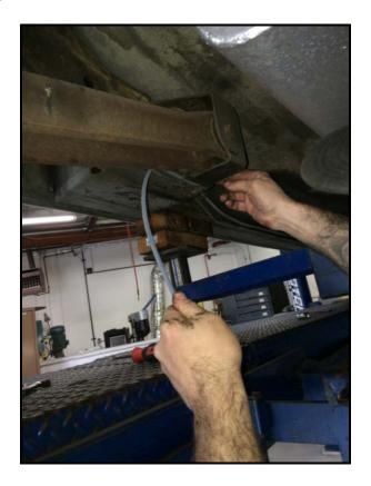
3 Unbolt the Front and Rear Bushing Mounts
