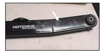
12) Check that all hardware is in place and tightened. Cover the zerk fittings using the plastic caps provided. Use a jack to remove the jack stands, and you're finished installing your new arms!
