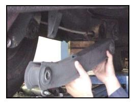
6) Using the grease provided, **apply a heavy coat of grease to the sides of the bushings** at both ends. Apply a light coat of grease to the surface contact areas of the bushing on the frame and axle too.
