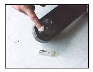
7) With the bushings greased, install the arm into the mounting locations on the frame and axle. Use the hardware kit provided to secure the Hotchkis trailing arm in place. **Do not** tighten the hardware until both ends have been connected to the axle and frame.
