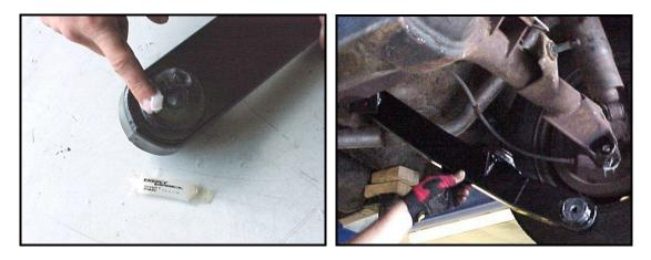
7) Install the arm into the mounting locations on the frame and axle. Use the hardware kit provided and the original shock mount stud to secure the Hotchkis trailing arm in place. **Do not** tighten the hardware until both ends of the arm have been connected to the axle and frame.
