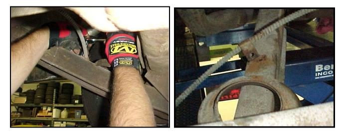
3) Unbolt the shock from the rear axle, and pull it clear of the mounting stud.
