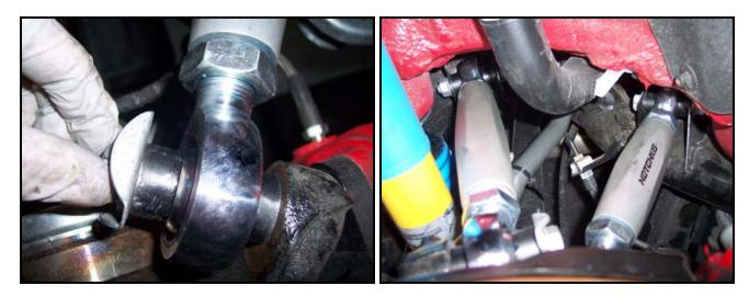
6. Tighten all of the control arm bolts, and use the supplied zip-tie to attach the ABS line to the upper control arm.
