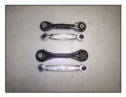
5. Install the new arms into the car. The shorter arm goes towards the front of the vehicle. Note that one rod end spacer on each arm has a tapered end. Make sure to install the tapered end against the suspension upright.
