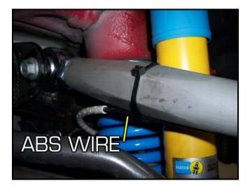
7. Make sure all the nuts & bolts are fully tightened. An alignment must be performed after installation is complete.
