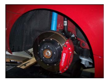
2. Remove the ABS wire retaining clip from the upper control arm.
