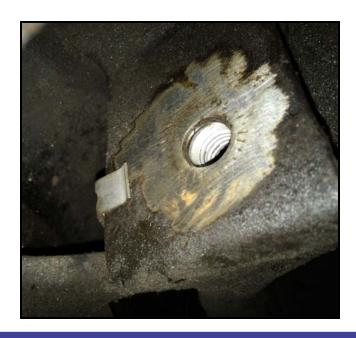
Once you have clean these areas. Grease the bushings outer surfaces with the provided silicon grease. You can also grease the frame/rear end surfaces that you just cleaned.
