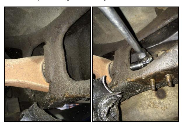
4 *Unbolt the Rear Mount*Unbolt the rear mount of the rear upper trailing arm.
