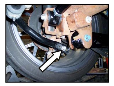
3. Disconnect the rear lower shock mounts on the both sides.
