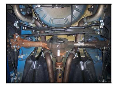
2. Disconnect the sway bar ends from both sides.
