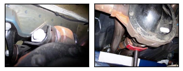
11. Reconnect the lower shock mounts and sway bar.
