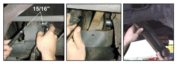
3) Check the stock arm mounting hole center-to-center measurement. The Hotchkis upper arm center-to-center length should match the stock arm measurement.
