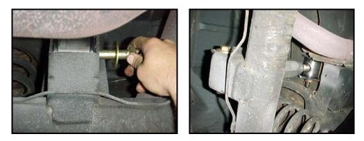
6) With the arms in place determine if any pinion angle adjustment is necessary. <u>For stock</u> <u>vehicles no adjustment should be required</u>, and you may move on to step 7. If the pinion angle needs to be adjusted downwards the arm length needs to be shortened. If the angle needs to be adjusted upwards the arm length should be lengthened.
