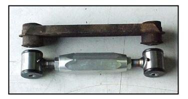
If the Hotchkis arm does not match the center-to-center length of the stock arm then you should adjust the length to match. Loosen the jam nuts at each end and turn the **center** section only! <u>Do not</u> turn the ends individually, as this will shorten the range of adjustment for the arm. Loosely tighten the jam nuts against the center section to hold it in place for the installation.
